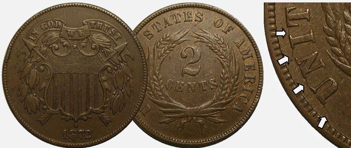
1872 two-cent piece, showing reverse die crack
